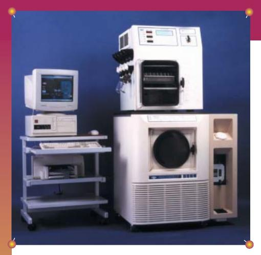
VirTis Freezemobile 35XL Series Freeze Dryer with pump module and LabTop with one shelf; computer workstation with wizard software. Wizard control system on LabTop.
