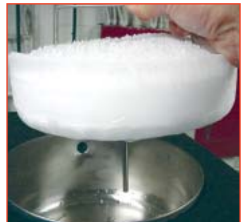
Shelf also serves to rapidly remove the collected ice when manifold drying.
