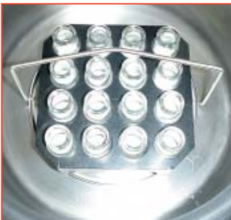
Shelf handle allows lowering the shelf for rapid vial freezing.
